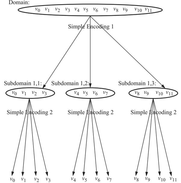
Figure 2. Example of a hierarchical, recursive, and hybrid encoding. A domain of 12 values,  $\{v_0, v_1, \dots, v_{11}\}$ , is divided into three subdomains by Simple Encoding 1 at level 1. Each subdomain is further divided into four parts by Simple Encoding 2 at level 2, where each part is a different domain value.
