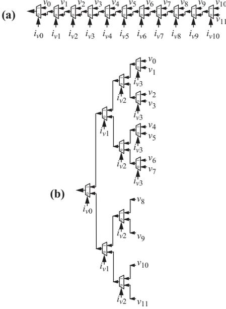
Figure 1. Two structural SAT encodings based on ITE trees for CSP variable  $v$  with domain of 12 values,  $\{v_0, v_1, \dots, v_{11}\}$ : (a) ITE-linear; and (b) ITE-log. ITEs are shown as multiplexors. In general, the ITE tree for a CSP variable can have any structure.
